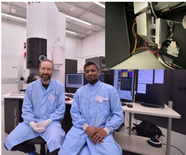
Figure 9 Olivier and Sharath with the Themis at Uppsala University. The CEFID filter, mounted under the TEM is shown in the inset with its 90-degree prism.
